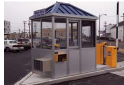
7'x5' Duraluminum with standing seam pitched roof, bullet resistant construction and custom top-suspended transaction window.
